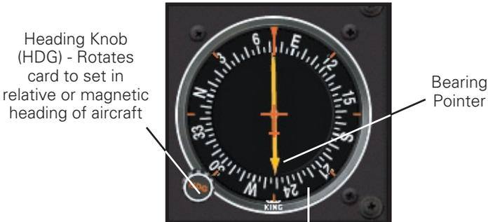
Compass Card - Manually rotatable card that indicates relative or magnetic heading of aircraft, as selected by HDG knob.
