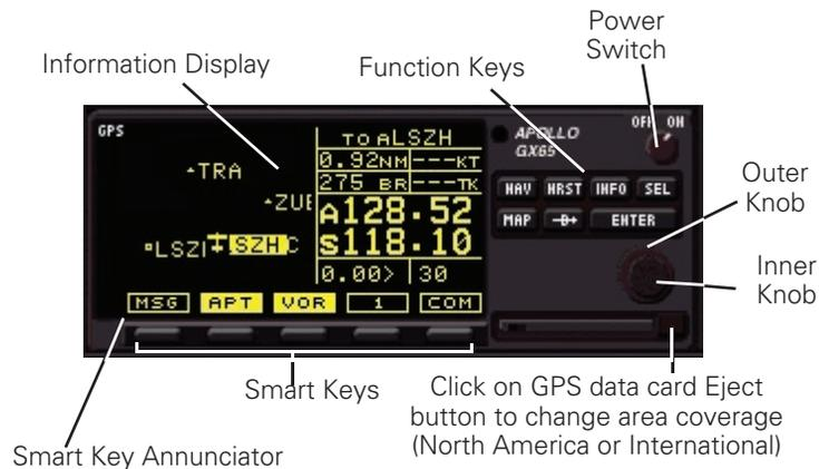
The Apollo GX products are high performance GPS products with a high resolution moving map display. The Apollo GX's use a powerful, accurate 8-channel GPS engine designed specifically for high performance aviation use.
