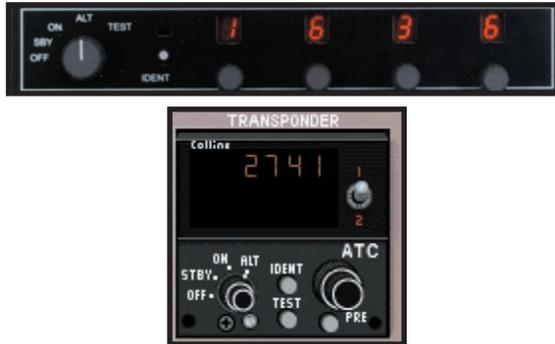
The transponder radio may be programmed to hold a pre-selected squawk frequency as well. Simply depress the PRE button for two seconds and then dial in the desired squawk code with either the mouse or by using the four control knobs on the AP3000. When done depress the PRE button again. This will save the desired code and may be retrieved at any time simply by pushing the PRE button.
