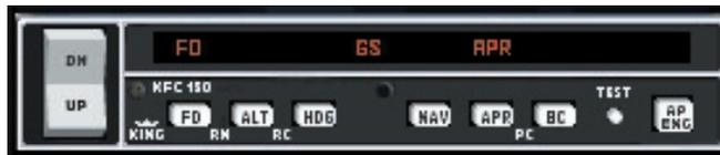
The KFC 150 and KAP 150 are both two-axis automatic pilot systems that operate almost identically. These autopilots each provide pitch and roll stabilization and automatic trim as well as automatic response to all selected autopilot modes. The only difference being the KFC 150 also has a flight director (FD) function. Since the KAP 150 does not have a FD function it uses a standard attitude reference without V-bar commands.
