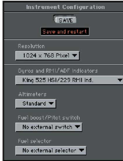
Instrument Configuration panel of A36 Bonanza
