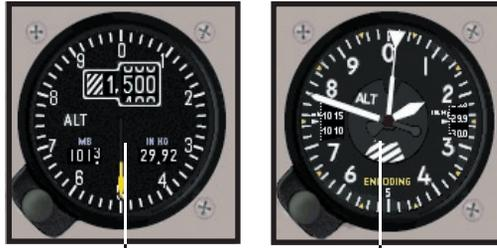
Choose between standard or digital altimeter (see Sec. III, Instrument Configuration)
