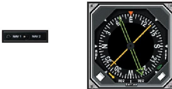
The NAV1 NAV2 toggle allows the user to switch the yellow needle of the RMI between VOR and ADF. The green needle requires the mouse to switch between VOR and ADF.
