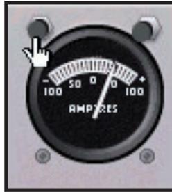
The amp meter shows charge or discharge information. Check generator load by pressing left or right engine AMP button.
