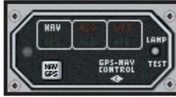
GPS navigation using the autopilot may be accomplished by first selecting the desired navigational fix on the Trimble GPS, then pressing the NAV GPS button on the GPS-NAV CONTROL box located above the Attitude Indicator and then pressing NAV on the autopilot.
