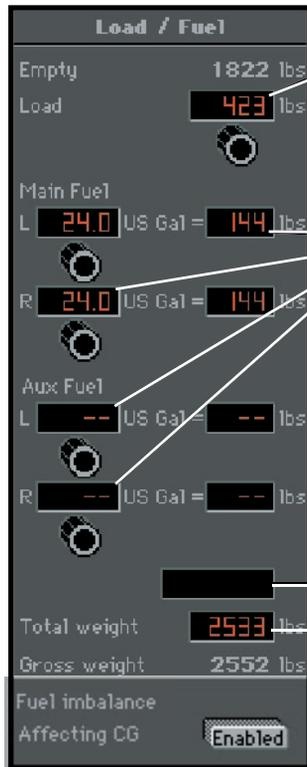
Set aircraft load weight (change from KGs to LBS. in **CONFIGURATION** page, under UNITS.
