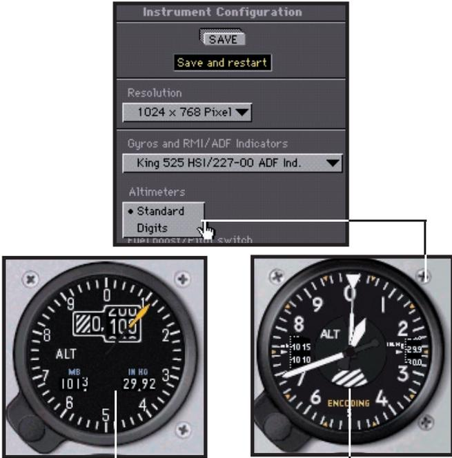
Possible changes to the avionics configuration and type of altimeters can be chosen on the Bonanza's **Configuration** Page
