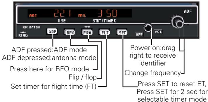
The Automatic Direction Finder Receiver (ADF) in **ELITE** selects a Non Directional Beacon (NDB) in the frequency range  $\pm 600$  Hz around the frequency set. This means that, for example, an NDB with a frequency of 371.5 kHz may be received with the ADF set to either 371 or 372.
