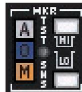
When passing a marker, the appropriate identification code is heard while the corresponding marker lamp flashes. The duration of the
