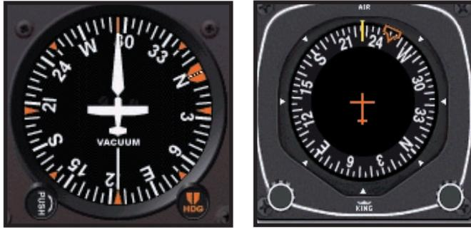
The orange arrow (heading bug) can be set with the rotary dial at the bottom right.
