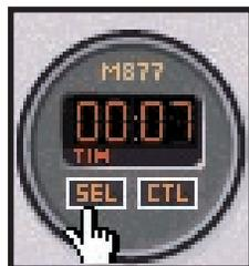
SEL button toggles between UTC, OAT and timer modes. When in the OAT mode, Fahr to Cen can be changed by pressing the **CTL** button. In the timer mode, pressing **CTL** will start or stop timer. Holding **CTL** for approximately 2 seconds will reset the timer to zero.
