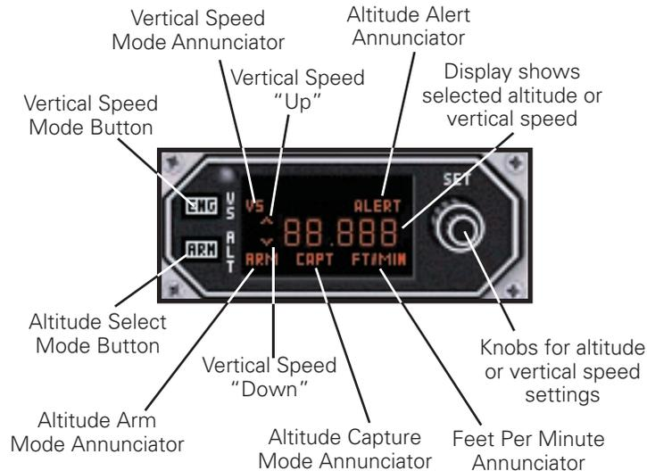
This feature is available only with the Bonanza, Baron, Seneca III and King Air (King radio option) aircraft modules only. The KAS 297B offers the user the ability to pre-select altitudes and vertical speeds while using the autopilot.
