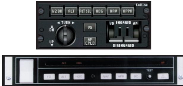
To use the Collins Flight Control System please note which functions are operated by which buttons on the AP 3000 avionics panel:
