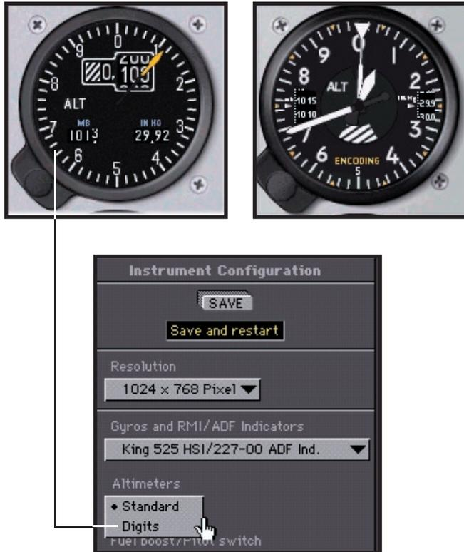
Possible changes to the avionics configuration and type of altimeters can be chosen on the Baron's **Configuration** screen. The standard configuration for the Baron 58 is the HSI and RMI. The **Configuration** screen allows you to change the avionics configuration: HSI with slaved ADF, HSI with non-slaved ADF, Directional Gyro (DG) with slaved ADF. When in the ADF (slaved or non-slaved) mode, click on the ADF instrument to change it to a VOR #2.
