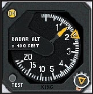
Radar Altimete, click on button to test or click and drag knob to set the Decision Height (DH) bug. The DH light on the radar altimeter and attitude indicator will light when designated height above ground is reached.
