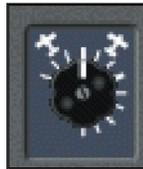
The rudder trim knob is only functional when used in conjunction with rudder pedals or if the Yaw Control feature is 'Enabled' on the CONTROL Page. If the Yaw Control is 'Disabled' the ELITE software locks out the rudder trim and the aircraft maintains coordinated flight.
