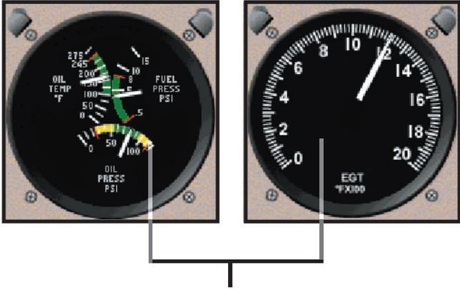
To change the engine oil temperature/oil pressure/fuel pressure tri-gauge to the EGT gauge simply click on the center of the instrument. Toggle back in the same manner.
